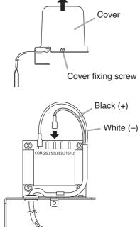
25 Ω 50 Ω 83 Ω 167 Ω Line 60 W 200 W 120 W 100 V line 70 V line 200 W 100 W 60 W 30 W
